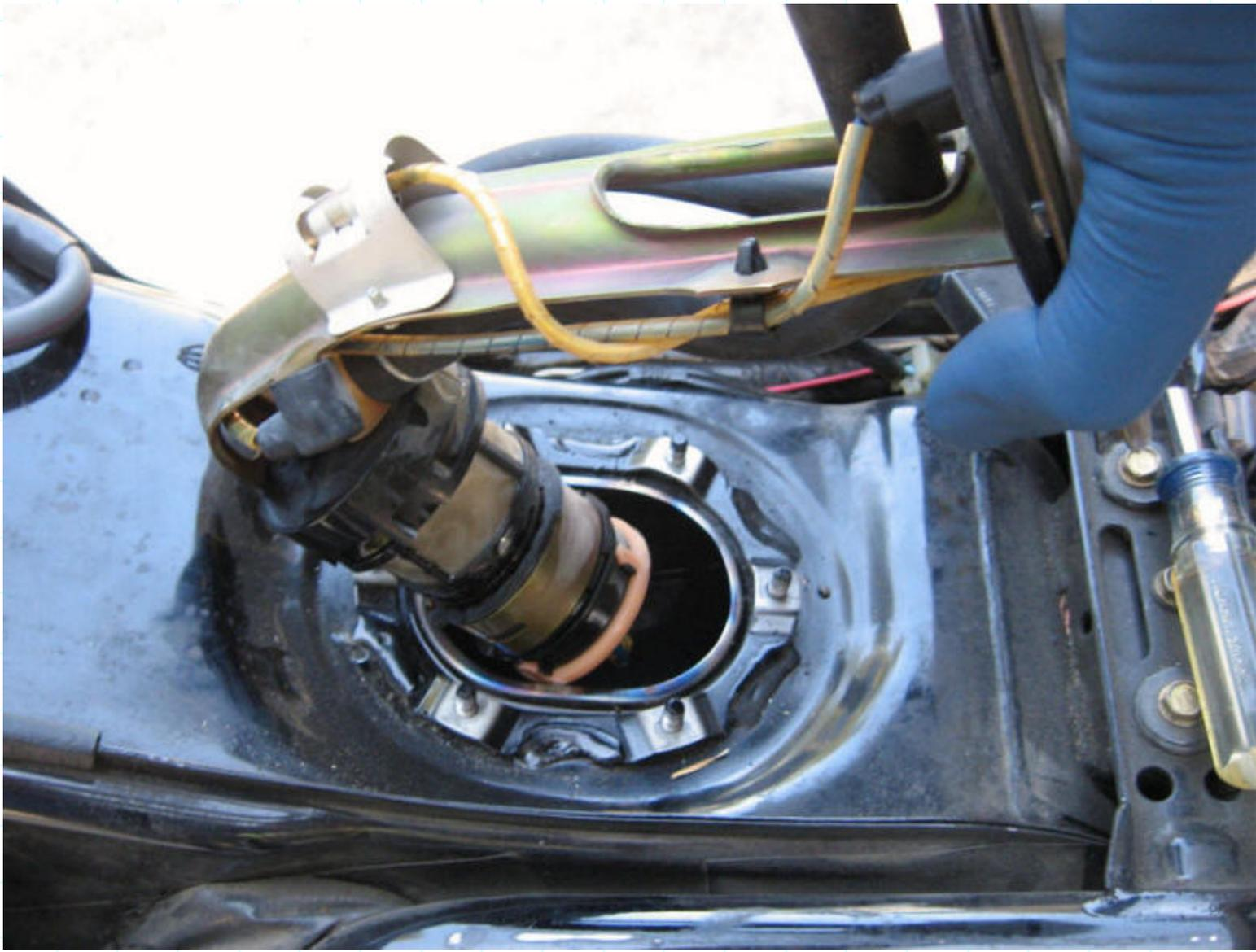
Now cut the 2 wires close to the pump and remove the hose from the fitting on the tank cover. Finally, remove the screw from the band clamp that holds the pump/strainer assembly and remove the assembly as shown (see pic).
